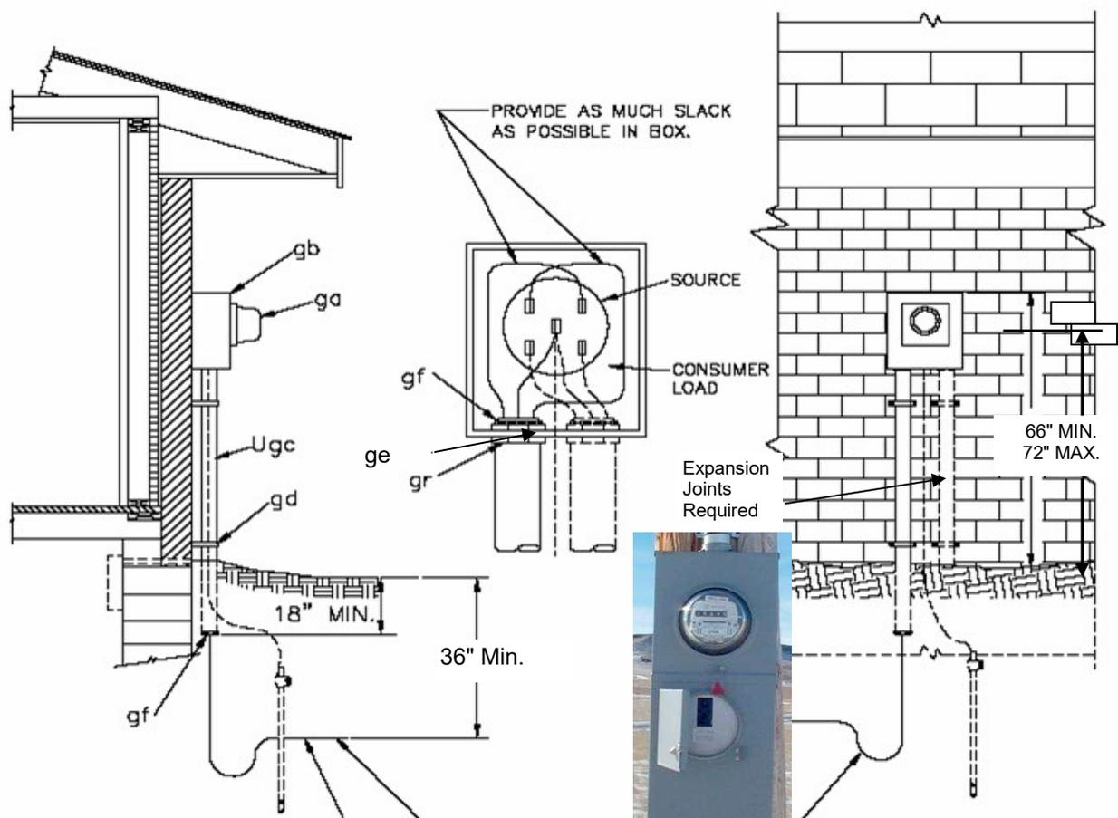
HAND TAMP, PREFERABLY WITH PNEUMATIC TOOL. BACKFILL WITH CLEAN MATERIAL.
