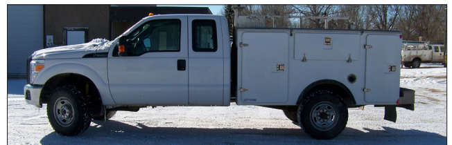
Unit 4071: 2016 Ford F-350 SuperdutyXL; 6.2L V8 gasoline engine; 4x4 automatic, extended cab
