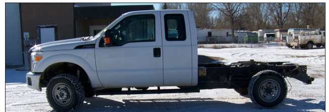
Unit 4064: 2015 Ford F-250 Superduty; 6.2L V8 gasoline engine; 4x4 automatic, extended cab, cab and chassis only
