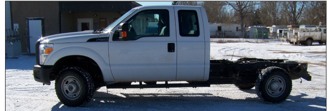
Unit 4034: 2015 Ford F-250 Superduty; 6.2L V8 gasoline engine; 4x4 automatic, extended cab, cab and chassis only
