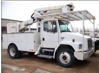
2001 Freightliner FL70 with TL41M Telelect aerial lift
